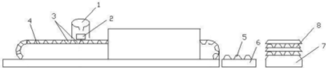
Figure 1- Casting conveyor for casting commercial magnesium
